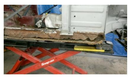
Removal of the splash panels presented some more surprises. We knew the bottom side members on both sides were rusted and had some holes, but we didn't know the inner panels were half gone due to rust. So the restoration began. Marsha and I did the removal and disassembly of the easy parts such as seats, carpet, radio, etc. Ron Kuhnau, Lyn Pond and Bruce Altman accepted the challenge to take on the rest of the restoration.
