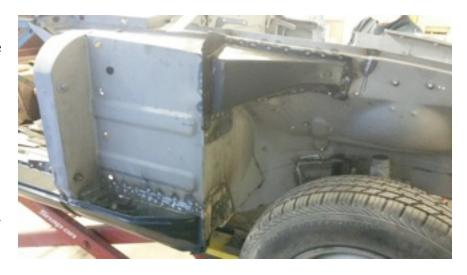
After a lot of cutting to remove the rusted parts, the new body parts were installed. Once this was completed the car was put on a trailer and taken to Highland Community College to complete the body work which included patching, sanding, priming and finally painting. The car is being painted Snapdragon Yellow, not it's original color which was Damask Red. We are at the painting stage as you can see from the pictures.
