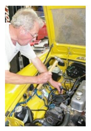
DO NOT POKE A HOLE IN THE OIL FILTER; you will end up with oil all over Hades when you try to remove it with oil running out of the bottom and the top of the filter.
