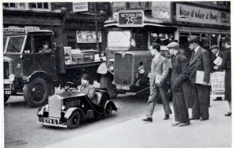
HE LAUGHS AT BUDGETS: This midget car, with its 17-yr. driver, was seen in the West End last week. Measuring less than 5 ft. in length, with a 2½-h.p. engine, this car will do 90 m.p.g. and seems to be the perfect answer to the new h.p. tax
