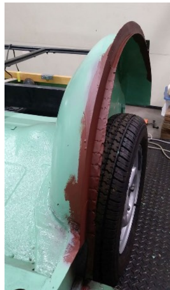
Welded and primered.
