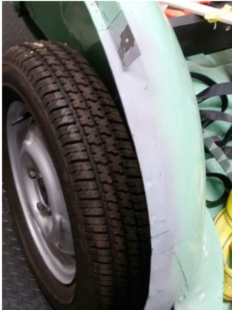
Before repairs, front section of flange trimmed
