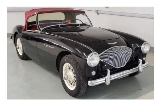
The first Austin-Healey 100s were designated BN1, employing the Austin 2655cc 4-cylinder engine and a 3-speed transmission with overdrive. Except for the first 20 cars, they were finished at Austin's Longbridge plant. The BN2 replaced the BN1 in 1955 and offered a 4-speed transmission as well as optional two-tone paint.
