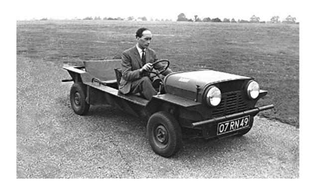
The Mini Moke was also originally targeted as a lightweight military vehicle, but the small wheels and low ground clearance and made it unsuitable for off road use. Shifting to the backup plan the design was offered to the civilian world as a lightweight, easily maintained, recreational and utility vehicle. Success was all but assured when Brigitte Bardot was photographed driving one.
