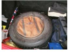
check the pressure and condition of that tire before going forward. If the tire needs replacement, now is the time to do it. I think the spare tire is probably the most neglected replacement part of the entire car. After checking out the tire, place the tire and wheel upside down over the attachment fixture on the trunk floor. You will need to make a small metal or wood plate and drill a 3/8" hole in it. Get a 3/8-24 bolt about 1 ¼ long and fasten the tire and wheel to the trunk floor.
